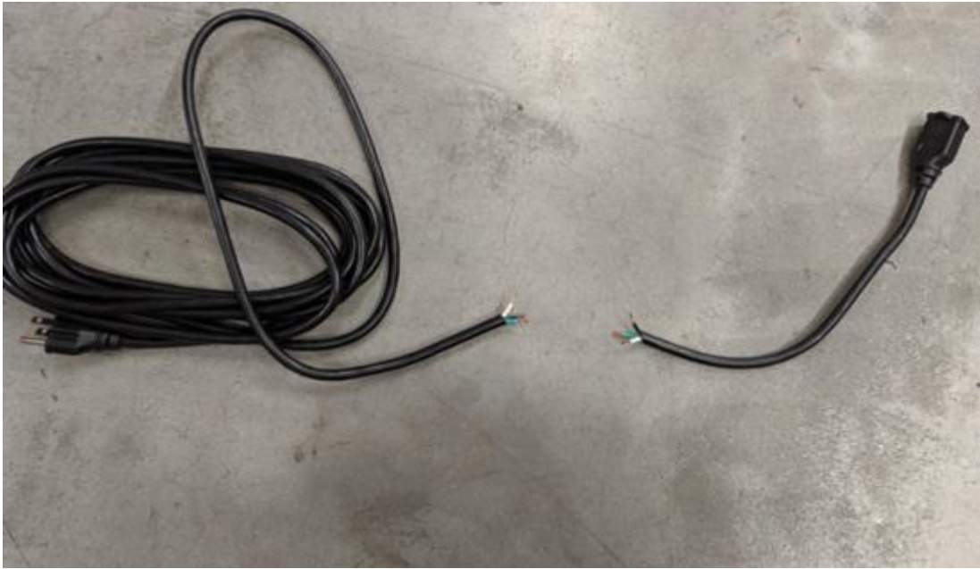
Figure 24: Location to Cut AC Extension Cord
