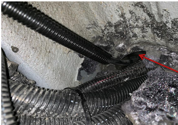
Figure 23: Front Grommet with Incision for Extension Cord
