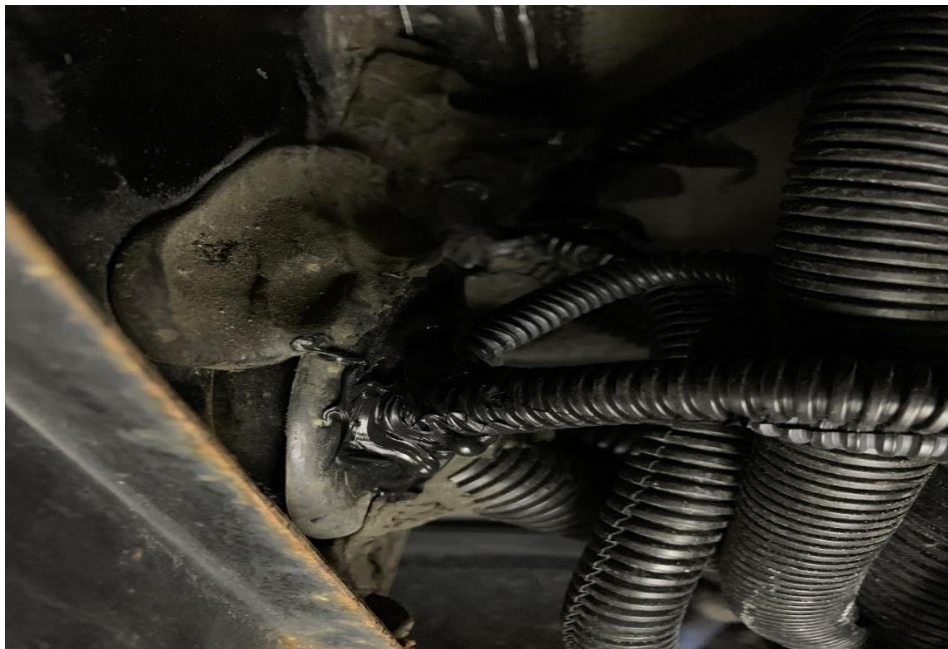
Figure 27: Loomed Wires Through Sink Grommet
