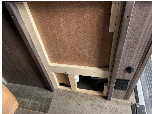
Figure 30: Interior battery pack access panel removed.
